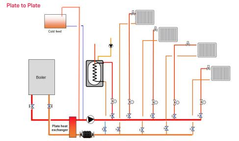
Note. For servicing, isolation valves need to be fitted either side of the filter. These valves are not supplied with the filter.
