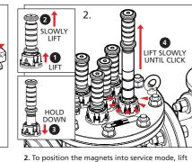
and hold the grey locking ring, then carefully pull up the magnet. After the magnet is released, hold down the locking ring and continue to slowly lift the magnet assembly until it locks into the service position. Ensure that the magnets are not removed from the filter completely
