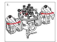
7. Re-open both isolation valves then refill the system as required. Bleed the air from the filter using the air vent. Ensure all magnets and pockets remain dry at all times. Remove any excess fluid from the top plate.
