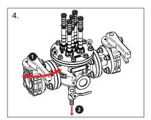
4. Partially open the inlet isolation valve, leaving the outlet isolation valve in the closed position and allow the deposits to drain through.
