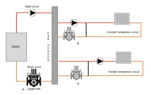
Installation with a Low loss header
