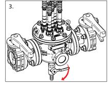
3. Connect a hose to the 11/4" drain valve or place a bucket underneath the unit. Open the drain valve or remove the drain plug.
