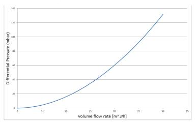
4" MagnaClean Pressure Differential vs Flow Rate
