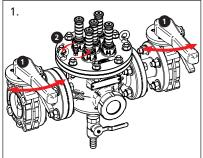
1. Check the MagnaClean sight glass for build-up of black iron oxide. Turn off the boiler and isolate the electrical supply prior to servicing. Turn off the isolation valves on either side of the product, then open the air vent located on top
