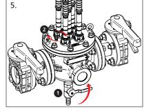
5. Close the inlet isolation valve once the water runs clear, then close the drain point by turning off the drain valve or replacing the drain plug. Close the air vent
