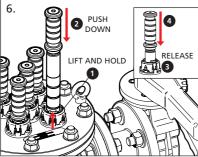
6. To replace the magnets to operational mode, life and hold the grey locking ring up and slowly push the magnet assembly down. Release the locking ring and continue to slowly push down the magnet assembly until it locks into operational mode. Repeat the procedure for each magnet assembly.
