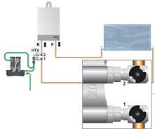
13 Add a suitable inhibitor, such as MC1+\*, into the canister. i.e. use the pro-fill bleed valve or remove canister lid assembly and dose filter. Open up the isolation valves and remove any air by venting using filter air vent.
