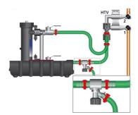
Turn OFF the HTV connector isolation valve 2 on the return pipe to the boiler, leaving the HTV isolation valve 1 open.
