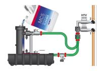
**6** Turn ON isolation valves on the RapidFlush Filter. Re-fill and pressurise the central heating system ensuring the radiators are half-full. Check for leaks.
